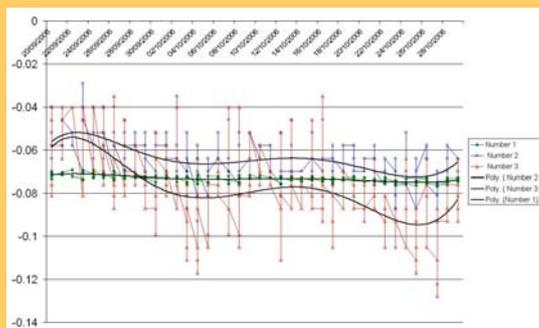
There has been no movement at Station 1, which follows a horizontal line. Station 2 shows some movement, and Station 3 even more.
